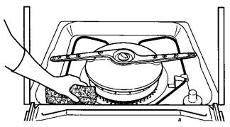
**Do not** clean the dishwasher interior until it has cooled. Wear rubber gloves. **Do not** use any type of cleanser other than dishwasher detergent because it may cause foaming or sudsing.
